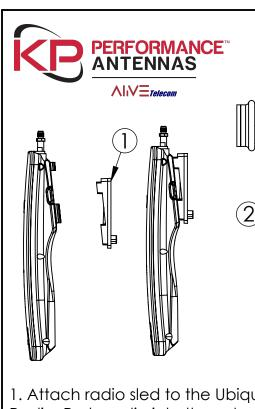
1. Attach radio sled to the Ubiquiti Rocket Prism Gen 2 Radio. Push radio into the adapter to lock into place. Slide tab button to release radio. **GPS Antenna Mount**
