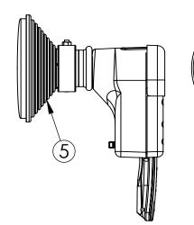
3. For horizontal/vertical polarization, align the radio to point updown. For +/- 45 Slant polarization, align the radio at a 45 degree angle.
