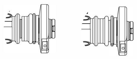
4. Pull back collar on Quick-Connect Waveguide Coupler and slide adapter over feed assembly. Release coupler.
