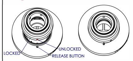
1. Attach Ubiquiti radio to adapter and align larger, UNLOCKED indent with radio's RELEASE BUTTON. Slot in adapter and rotate to smaller, LOCKED indent. To remove radio, press RELEASE BUTTON and rotate adapter to UNLOCKED indent.
