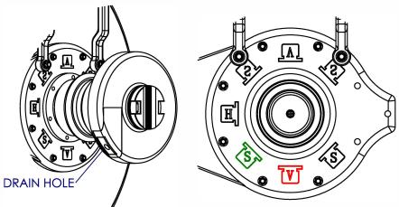
3. Rotate adapter such that orientation of radio's DRAIN HOLE is directed down. For Horizontal/Vertical polarization, align release button with antenna's bottom V indicator. For +/-45 Slant polarization, align release button with antenna's bottom left S indicator.
