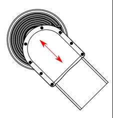
3. For horizontal/vertical polarization, align the radio to point up-down. For +/- 45 Slant polarization, align the radio at a 45 degree angle.
