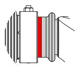
4. Pull back collar on Quick-Connect Waveguide Coupler. Slide adapter over feed assembly. Release collar to lock into place.
