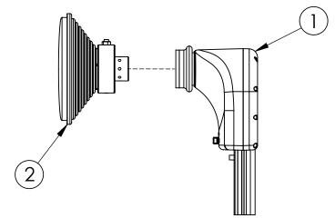
2. Align assembled radio adapter with feed assembly's input waveguide.
