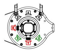
Align adapter with feed assembly's input waveguide. Rotate adapter such that direction of connectors is aligned with **H/V** (Horizontal/Vertical) or **S/S** (+/- 45 Slant) indicators on the back of the antenna.
