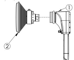
2. Align assembled radio adapter with feed assembly's input waveguide.
