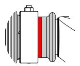
4. Pull back collar on Quick-Connect Waveguide Coupler. Slide adapter over feed assembly. Release collar to lock into place.
