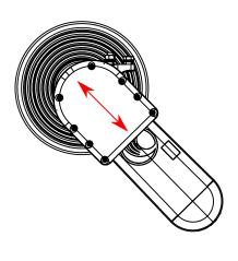
3. For horizontal/vertical polarization, align the radio to point up-down. For +/- 45 Slant polarization, align the radio at a 45 degree angle.
