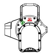
Align adapter with feed assembly's input waveguide. Rotate adapter such that the radio is aligned with the V (Horizontal/Vertical) or S(+/-45 Slant) indicators on the back of the antenna.
