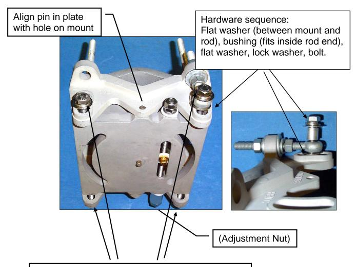
Confirm that the Mount is centered as shown. Use the flat washer, lock washer and nut for each lock bolt. (4X) Tighten securely.
