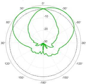
Three KPPA-3S3S-65SA mounted around a tower give complete coverage, at full sector gain.
